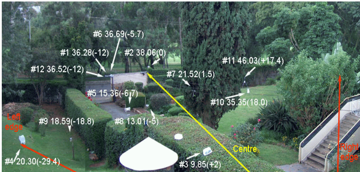
Figure 2 Placement of the transponders as viewed from the radar antennas
